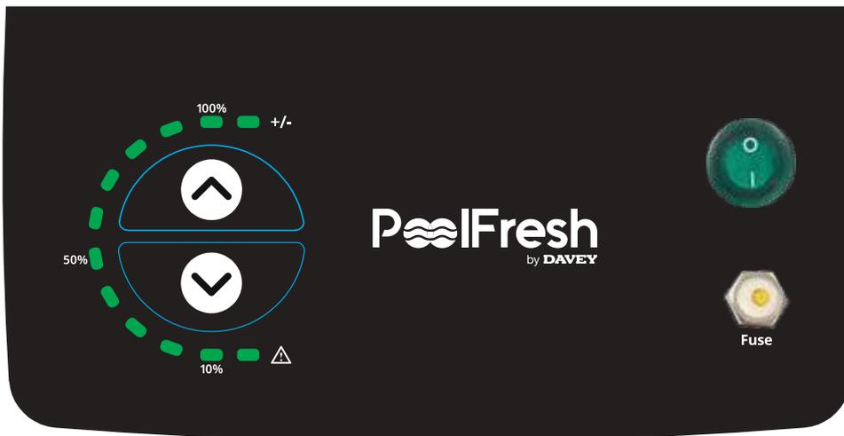
Once the salt level in the pool is correct the unit may be switched On. **(Note: Once the unit starts there is a short time delay until the cell operates to ensure filtration system is primed with water)** At this point the **Operation LED** should be Green; if red refer below. Once the unit is powered ON, some LEDs quickly ramp up to the last output set point. During normal operation, pressing the ↑ button increases the output set point and ↓ button decreases the output set point.
