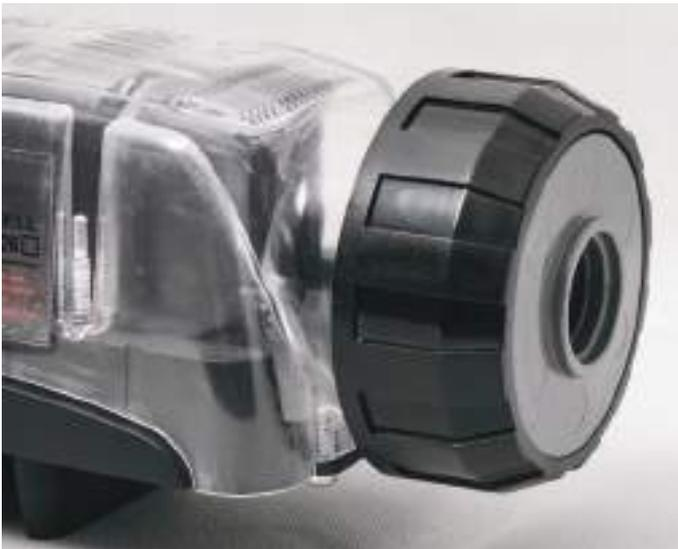
3. Secure the Cell in a vertical position with the blanking cap at the bottom, to catch any spills the Cell should be placed in an acid proof container.
