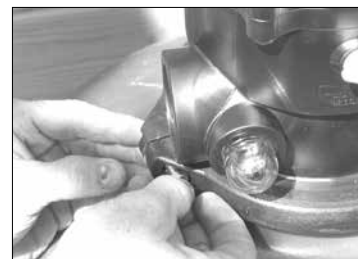
The 6-way valve is now placed on the filter and the clamp is fixed around the filter. This is how the valve is connected to the filter.
