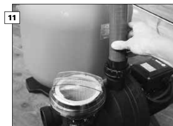
Screw the connector pieces into the filter and the pump. Slide the fittings and the inserts over both ends of the hose. Connect the fittings to the connector pieces, and then tighten the fittings. (see the technical section: 2.4.3 Connections)
