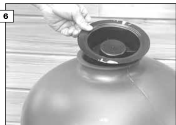
After filling the filter, remove the residue of sand at the top of the filter and remove the funnel.
