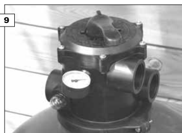
Unscrew the little valve at the side of the valve to fit the manometer.
