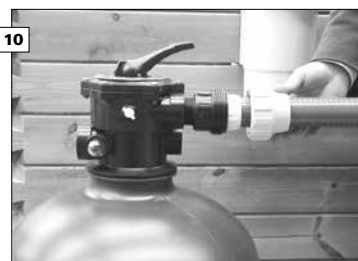
The pump and filter are interlinked by a semi-flexible tube.
