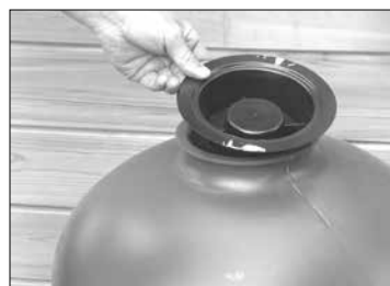
Make sure that the plastic protection (funnel) is placed on top of the filter to prevent sand/gravel from falling into the mouthpiece of the branch pipe.
