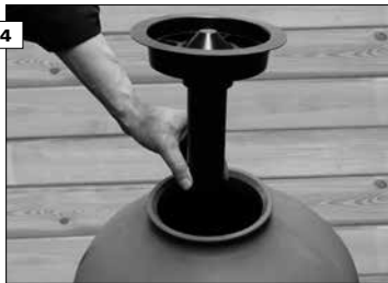
4 Make sure that the plastic protection (funnel) is placed on top of the filter to prevent sand/gravel from falling into the mouthpiece of the branch pipe.
