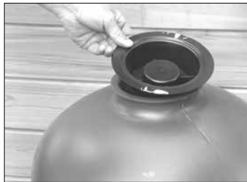
4 Make sure that the plastic protection (funnel) is placed on top of the filter to prevent sand/gravel from falling into the mouthpiece of the branch pipe.
