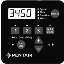
Figure 12: Setting Speed for Quick Clean
